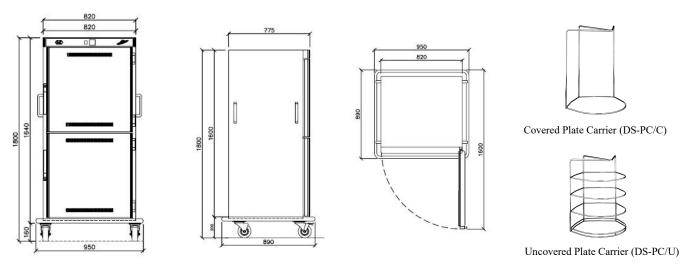
Notes: (1) The unit comes with 4 chrome plated shelves as standard. (2) Plate carriers are optional. Each plate carrier holds 4 pre-plated meals with a plate sized in 254mm in diameter maximum. 24 plate carriers are needed for a full capacity.
