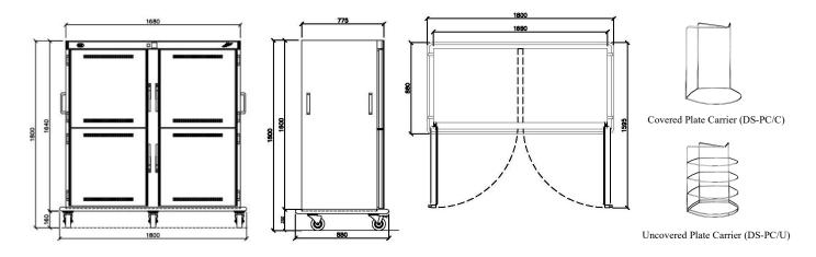
*Notes: (1) The unit comes with 8 chrome plated shelves as standard. (2) Plate carriers are optional. Each plate carrier holds 4 pre-plated meals with a plate sized in 254mm in diameter maximum. 48 plate carriers are needed for a full capacity.*
