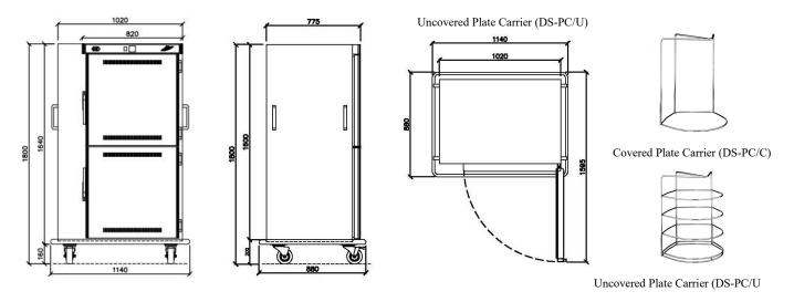
Notes: (1) The unit comes with 4 chrome plated shelves as standard. (2) Plate carriers are optional. Each plate carrier holds 4 pre-plated meals with a plate sized in 254mm in diameter maximum. 32 plate carriers are needed for a full capacity.
